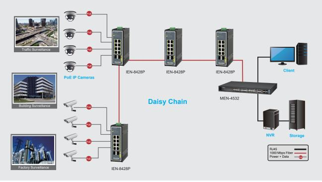
The IEN-8428P is compatible with 10/100/1000Mbps through RJ45 transceivers to guarantee a strong, stable connection of Ethernet, Fast Ethernet or Gigabit Ethernet, providing flexible deployment options to satisfy industrial Outdoor networking requirements. PoE IP Camera **Power Supply** (SDR-480P-48) **IP Camera** Power Line Alarm Relay PoE Power + Data Wi-Fi AP Control Cei 1000 Mbps Fibe NHL-28152
