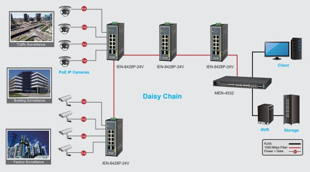
The IEN-8428P-24V is compatible with 10/100/1000Mbps through RJ45 transceivers to guarantee a strong, stable connection of Ethernet, Fast Ethernet or Gigabit Ethernet, providing flexible deployment options to satisfy industrial Outdoor networking requirements. PoE IP Camera **Power Supply** (SDR-480P-48) **IP Camera** Power Line Alarm Relay PoE Power + Data Wi-Fi AP Control Cei 1000 Mbps Fibe NHL-28152
